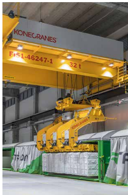
Konecranes' fully automated cranes loading pulp units into the train wagons.
